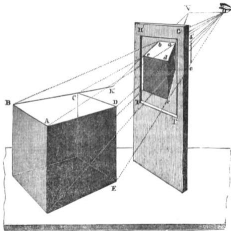
Figure 1. An illustration of the geometric principles underlying Alberti’s window, from Brook Taylor’s *Principles of Linear Perspective* (London, 1835). The viewer sees the 3D box as a 2D virtual object through a cropped window onto which the light rays from the box project through straight lines.
